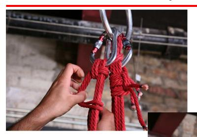
Pull on the working end to tighten ...
